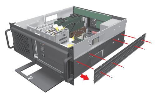
Figure 5. Removing Side Panel
